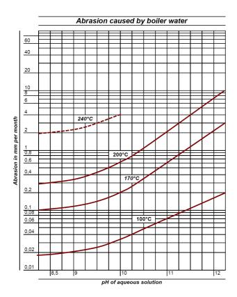
Glass loss - shown here for unprotected borosilicate glasses. The glasses life depends not only on the temperature but also on the water pH (higher pH values shorten glass life).
